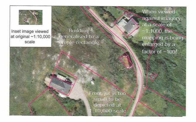
This image is an example of OS 1.10 000 detail (red lines) with the aerial imagery showing underneath.
