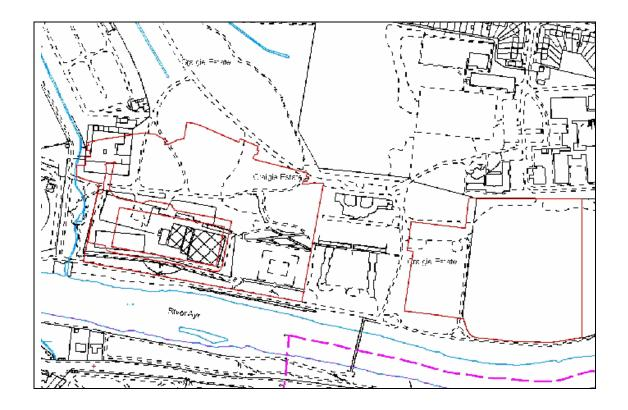
The polygons in red against OS background have been extracted from the CAD and imported to the DMS.
