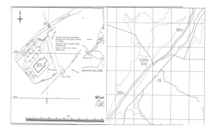
In this example the deed plan, although showing little surrounding detail would appear to be a reasonably good quality deed plan, prepared at a suitable scale for the detail it is depicting.
